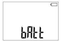
Batteries / rechargeable batteries fully discharged.
